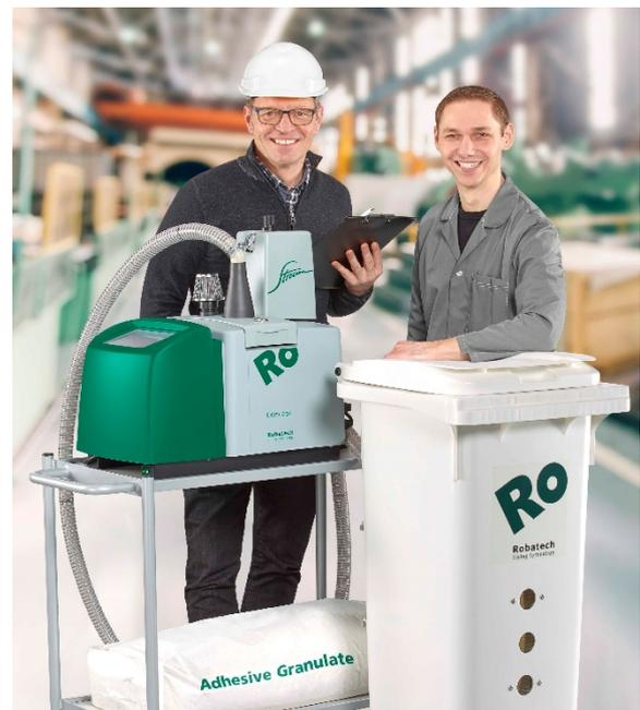
In particular, filling a hot melt adhesive system involves a certain risk, as the tank systems can reach temperatures of up to 200 °C. When opening the tank for filling, there is a risk of burns due to adhesive splashing or contact with already melted adhesive. These risks can be avoided with an automatic filling system.
