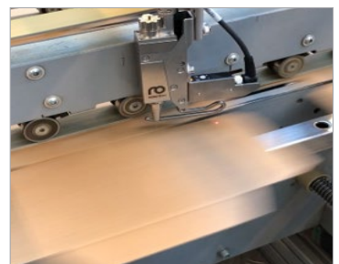
Application of SpeedUp creaser liquid to the fold line
