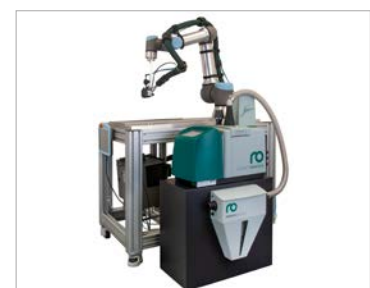
Cobot with adhesive application system and automatic filling
