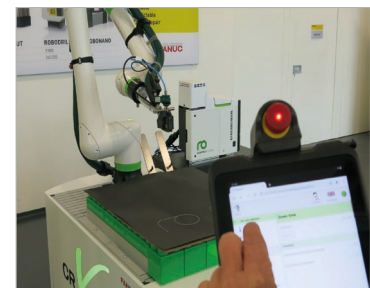
Cobot with adhesive application system and web-based visualization
