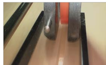
Precise placement of the tear strip
