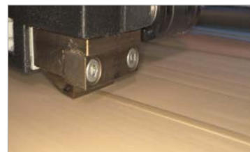
Uniform adhesive application accurate to the millimeter
