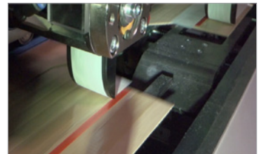
Precise placement of the silicone paper strip
