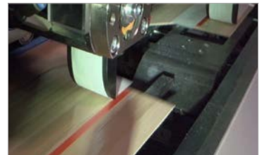
Precise placement of the silicone paper strip
