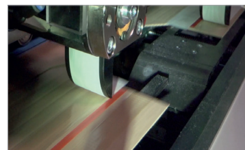
Precise placement of the silicone paper strip
