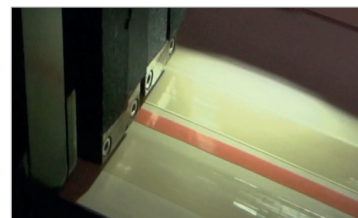
Uniform adhesive application accurate to the millimeter
