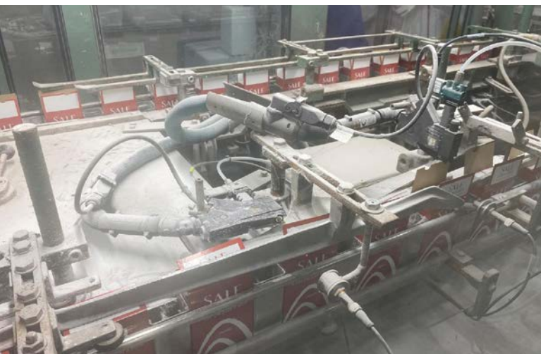
The SX Diamond spray head reliably applies adhesive beads even under harsh production conditions.
