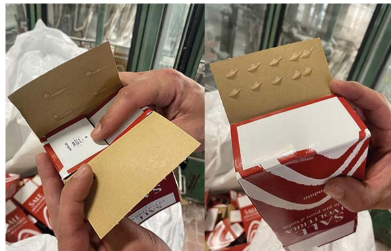
Adhesive application on the bottom flaps of the salt package.
