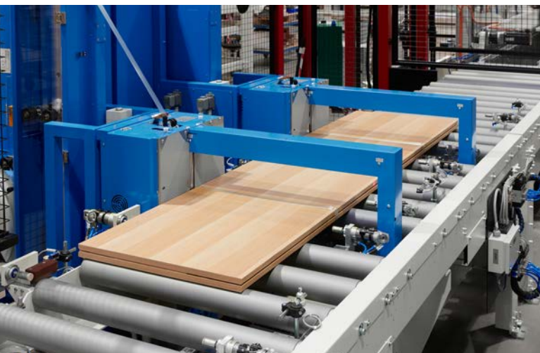
First step: The side panels are aligned together with the back panel
