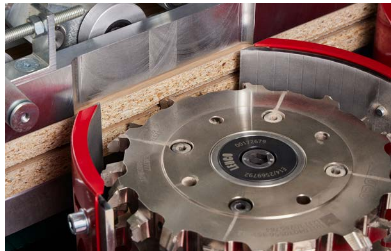
Second step: A precise joint is milled into the side walls
