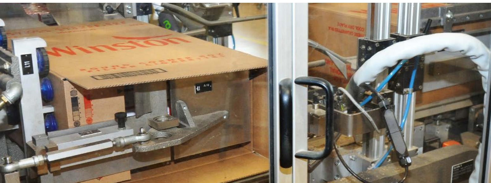
Cardboard flaps are folded (left) and then glued (right)
