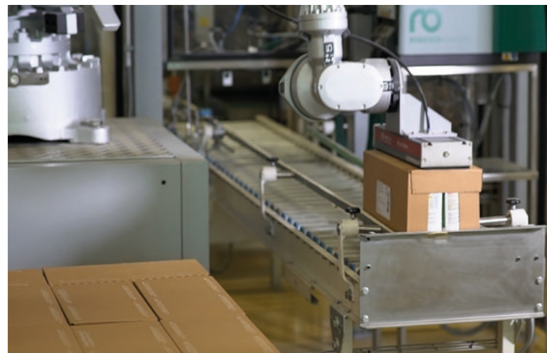
Palletizing secondary packaging with self-stick adhesive
