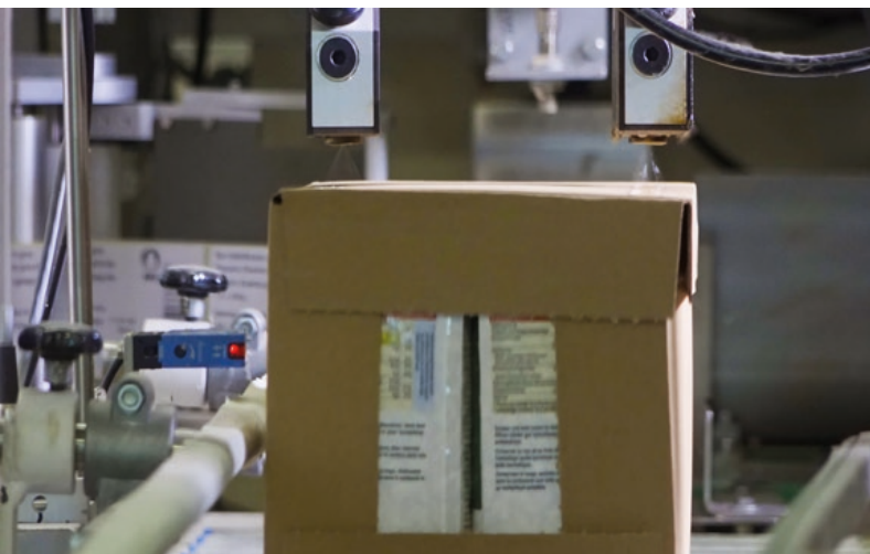
Two AX Diamond spray heads during adhesive application
