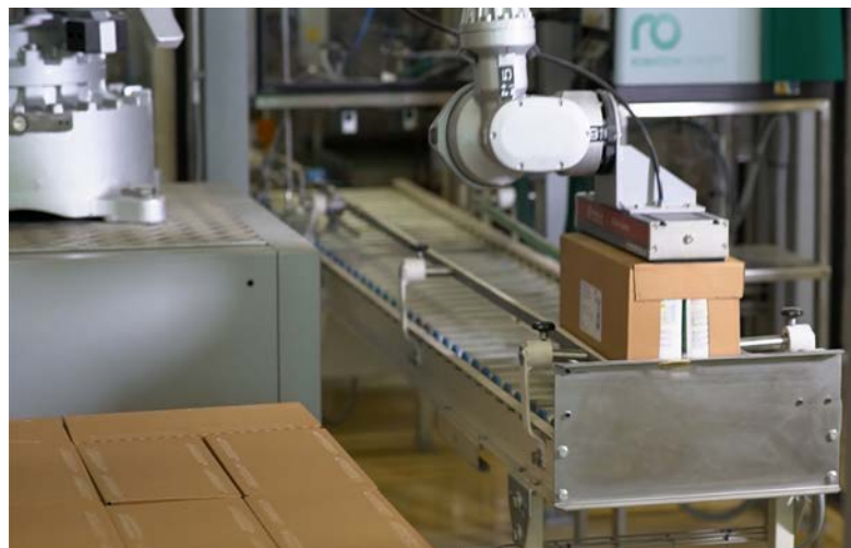
Palletizing secondary packaging with self-stick adhesive
