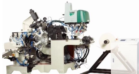
Dayuan paper cup machine with Robatech melter Concept (on top) and application head AX Diamond
