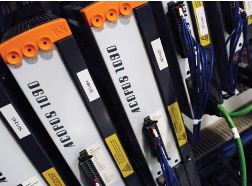
When it comes to utilizing servo drives to control the movement of its pick-and-place machinery, Pack-Smart prefers the modular ACOPOS servo drives supplied by B&R Industrial Automation.
